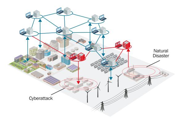
NREL is developing modeling capabilities to analyze and visualize the impacts of cyberattacks and natural hazards on the electric power system. For example, by co-simulating the grid and communications layers, researchers will better understand the interdependencies between infrastructure and find ways to optimize system architectures for resilience. Illustration by Anthony Castellano, NREL
